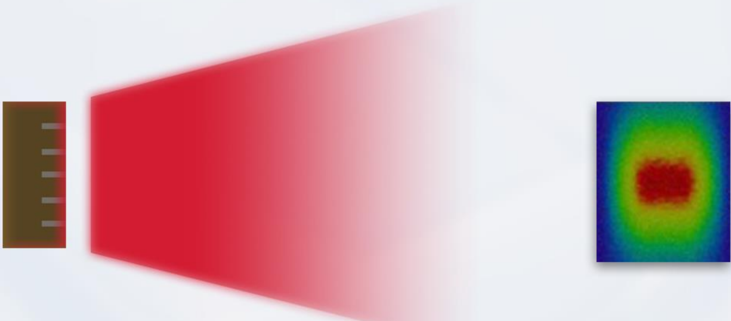
Without optical shaping, the beam diverges rapidly
